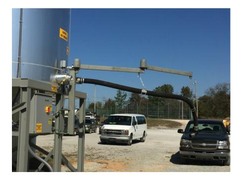
Especially designed with the spray patcher in mind. This makes it easy and clean to swing the hose over patcher to fill the tank.
