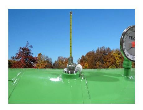
Emulsion level gauge lets you see how much emulsion in the tank with out opening lid or dumping the air pressure. By pulling the dip tape and catching the magnetic float you get an accurate fluid level.
